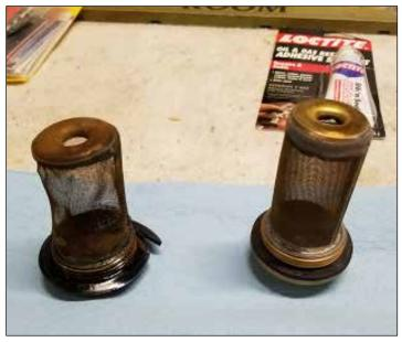
The old (left) and new drain plugs with attached mesh filters.
