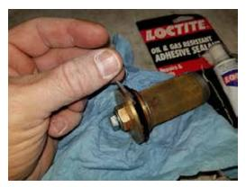
The failed gasket sealant.
